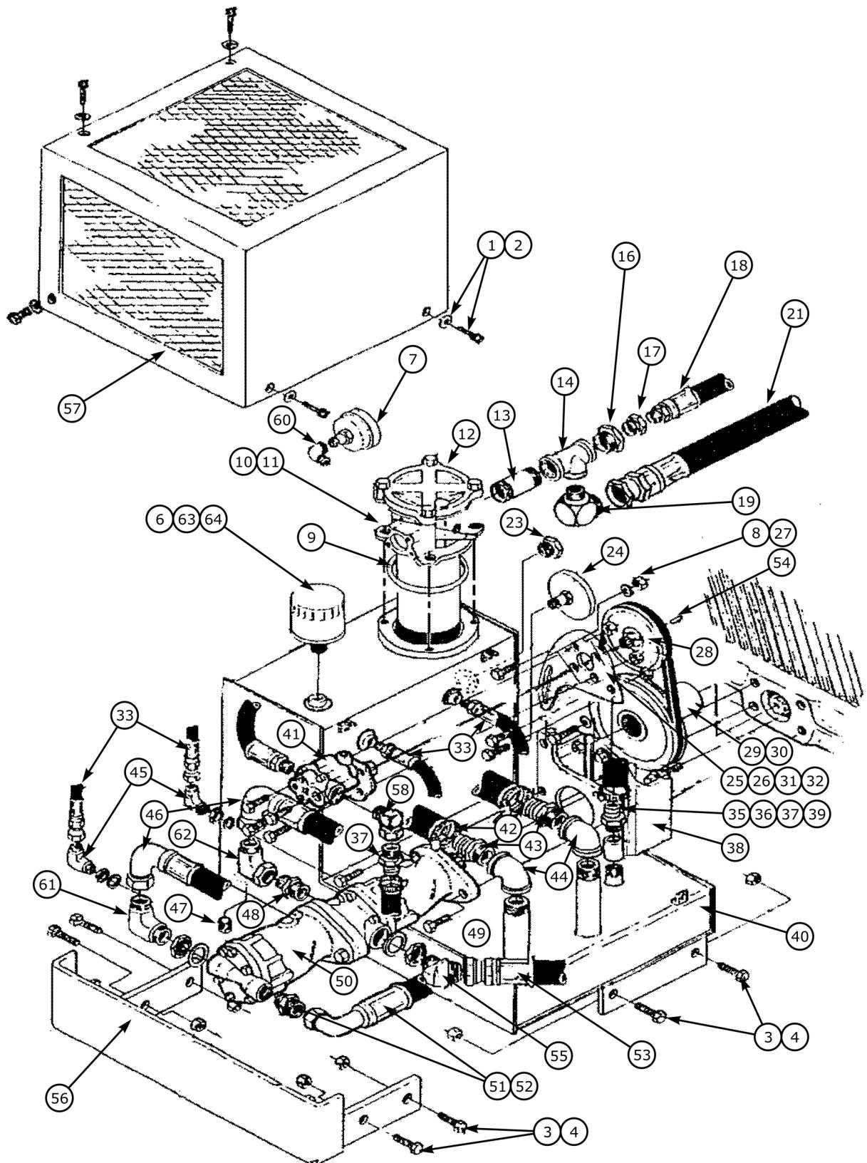
**PUMP & TANK ASY - TANDEM PUMP - DUAL WINGS (PART 2)**
